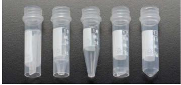
Maximum centrifugation RCF: 20,000g. (For Non-Skirted tubes only) Dimensions: 44 mm H x 11 mm dia.
