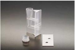
The Simport Double CytoSep™ Cytology Funnel with disposable sample chamber allows for two samples to be run simultaneously on a single slide and is ideal for immunohistochemistry work. The Double CytoSep™ Cytology Funnel provides a cell deposition area of 6 mm (28 mm squared) for sample volumes of up to 0.5 ml. The filter card comes pre-attached. Cap is included. No need to use a different stainless steel slide clip. Each component is also available separately.
