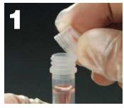
Screw Tamper Evident cap on tube until locking ring clicks over serrated tube neck.
