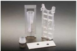
This CytoSep™ Cytology Funnel allows 2 sample deposition areas on a single slide. The disposable sample chambers do not need metal clips. Pre-attached filter card. This Sample Chamber is also disposable.
