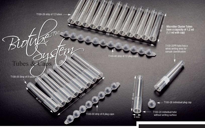
Tubes are made of autoclavable polypropylene and are available either individually or in strips of 8 or 12 detachable tubes. Tubes have a gross volume of 1.2 ml but with a cap in place, they will hold 1.1 ml.
