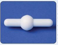
Many magnetic stirring bars can be impeded by powders in a liquid, but the newly-designed Saturn Spinbar® Magnetic Stirring Bar rises to this stirring challenge. A large sphere at the bar's center lifts the stirring bar ends while spinning and thereby reduces the surface contact area to allow the bar to spin with decreased drag.
