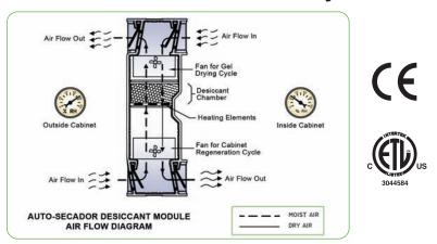
Module features color-changing, dustless, silica gel desiccant beads and two fans. Automatic dehumidification and desiccant regeneration cycle operates continuously every 20 minutes as follows:
