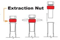
Safe-Lab<sup>™</sup> stoppers are easily removed from standard tapered glassware by turning the red extraction nut to apply a safe, gentle and even force against the mouth of the vessel, helping to eliminate accidents and breakage.
