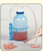
(¼" ID X ¾" OD), then connect the vacuum line to vacuum source and the aspirator is ready for continuous vacuum aspiration from Petri dishes, microtiter plates, flasks, centrifuge tubes. and more.
