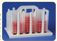
racks can be stacked together and interlocked to prevent accidental knock over. Finger access slots in the base allow a stack of dishes to be safely removed from the rack with a secure grip. Rack base is epoxy coated steel, and all other parts are made of white polypropylene. Steam autoclavable at 121°C (250°F). Racks are shipped flat and easily assemble in minutes.
