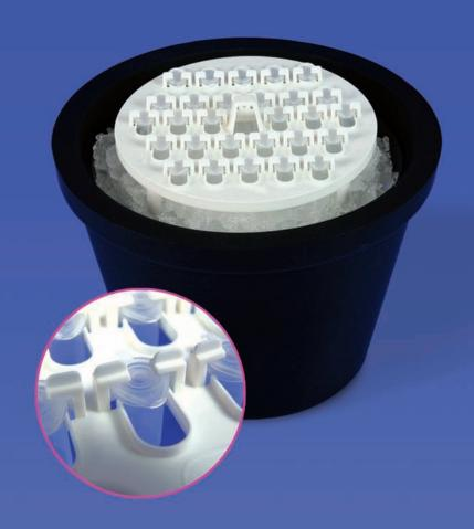
PrepSafe™ Floating Microcentrifuge Tube Rack
