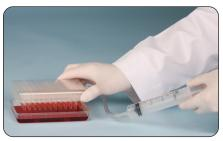
simultaneously changing media or the addition/removal of reagents from a 96 well plate. Made of transparent plastic material, it has a vacuum outlet at one end, and a short length of 3.2mm I.D. (%") tubing is supplied for syringe connection. Requires a 30ml or larger disposable sterile syringe (not included). Individually packed, available in Sterile/Disposable or Autoclavable/Reusable.
