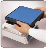
and carrying. Supports up to 6.8 kg (15 lb) and has a rotating orbit diameter of 1.52mm (1/16").
