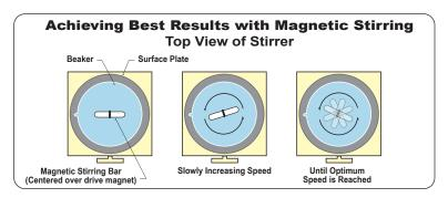
Vertical distance between the drive magnet and the stirring bar should be kept to a minimum for the best coupling and stirring efficiency. Therefore, the containing vessel should be as thin as practical.
