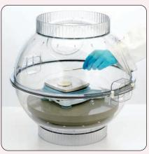
then close the cover to begin use. Two access ports allow maximum dexterity for sample handling and balance operation. The Damping Mount can be easily removed for cleaning or use outside the unit.
