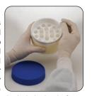
polyethylene vial holder that separates the vials from the isopropyl alcohol. A plastic foam insert surrounds the vial holder. Alcohol filled containers can be stored at room temperature. Universal symbols printed on the container show instructions for use.
