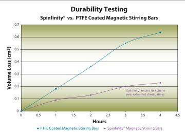
Spinfinity® and PTFE coated magnetic stirring bars were used under conditions known to cause material breakdown and measured for volume loss each hour for a period of four hours.
