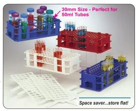
Each rack features end plates for labeling as well as numbered and lettered rows for tube identification. Interlocking feet allow stacking of racks for storage. Dimensions for all racks are  $24.6 \times 10.4 \times 6.4$ cm high ( $9.7 \times 4.1 \times 2.5$ ") and they assemble in seconds. Steam autoclavable at 121°C (250°F). **Per each, 8 per case.**
