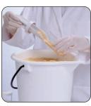
granular materials. A ribbed handle provides an excellent grip for pushing and turning the scoop. The depth and shape of the scoop keeps samples contained while allowing for easy dispensing into the clear styrene container. Supplied with labels for sample identification. F19856-0250 page 262 can be used to store and transport Samplit™ containers.
