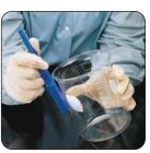
point where it can be grasped. The magnet is located in the  $25 \times 70$ mm (1 x  $2\frac{3}{4}$ ") rectangular section, and a long ribbed handle provides a secure grip. Made of high density polyethylene. Overall length: 20cm (7.7").
