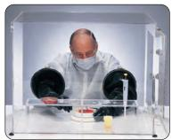
leveling. Gas purging of the glove box is possible via the supplied and easily assembled stopcock. Made of 6.35mm (¼") clear acrylic.
