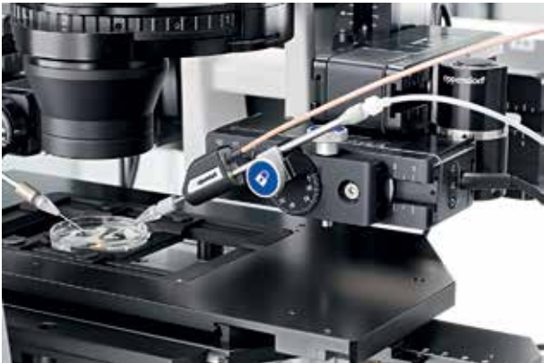
Eppendorf PiezoXpert actuator mounted onto TransferMan 4r
