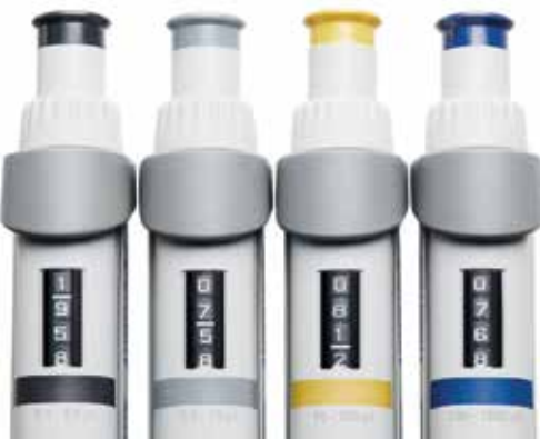
4-digit volume display to allow for more accurate volume setting.
