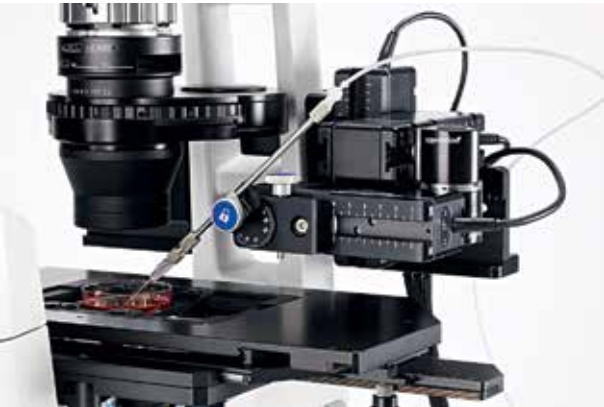
InjectMan 4 micromanipulator mounted for axial injection
