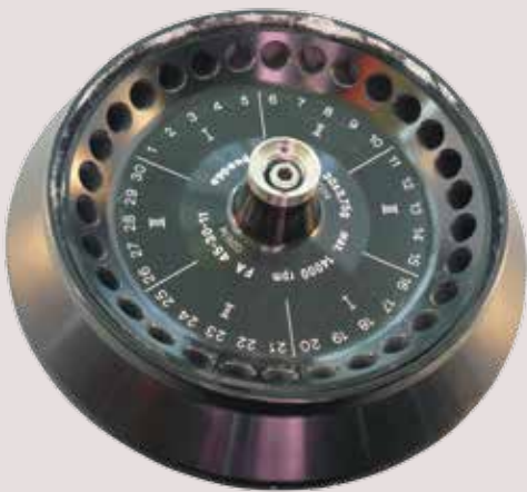
Rotor with “blistering” on the edge
