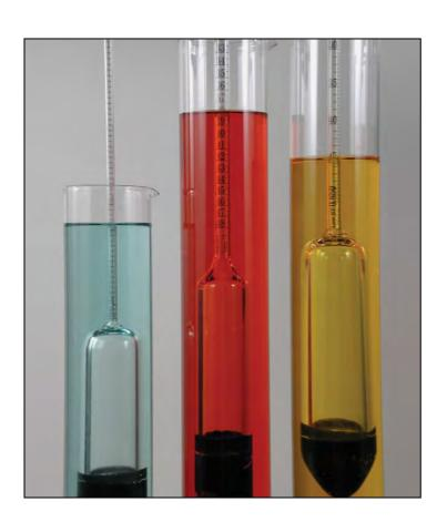
**Hydrometer Cylinders**These three hydrometer jars are available with a standard internal diameter of 37mm.
